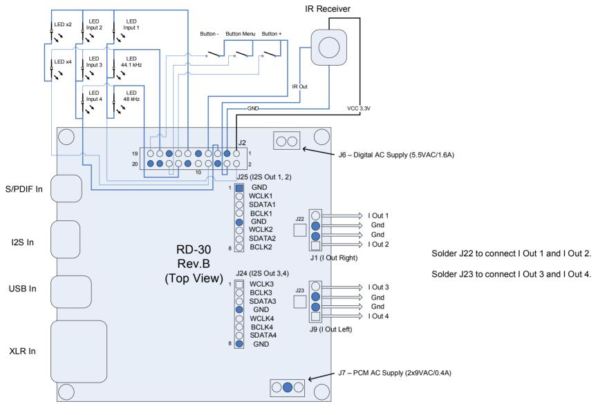
Place a jumper between J2 pin 10 and GND for differential output (4 Outputs X 1.2mA). With J2 pin 10 floating and J22 and J23 on DAC board soldered, output is single-ended with analog interpolation (2 X 2.4mA).
